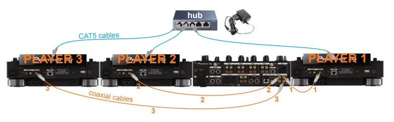
player digital out connected to the mixer digital input with digital audio cables [coaxial cables w/ RCA connectors]
