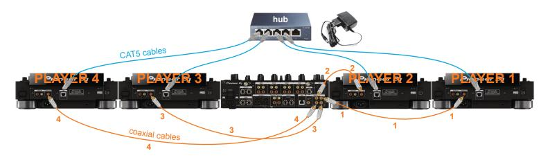
player digital out connected to the mixer digital input with digital audio cables [coaxial cables w/ RCA connectors]
