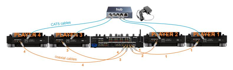
player digital out connected to the mixer digital input with digital audio cables [coaxial cables w/ RCA connectors]
